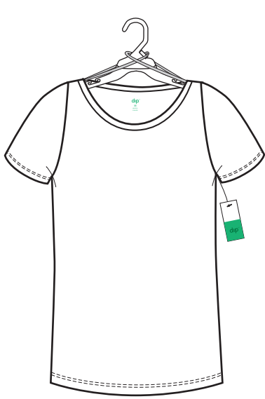
SHOULDER SEAM LOOPS ATTACHED TO INSIDE SHOULDER SEAMS AND LOOPED AROUND HANGER HOOKS
